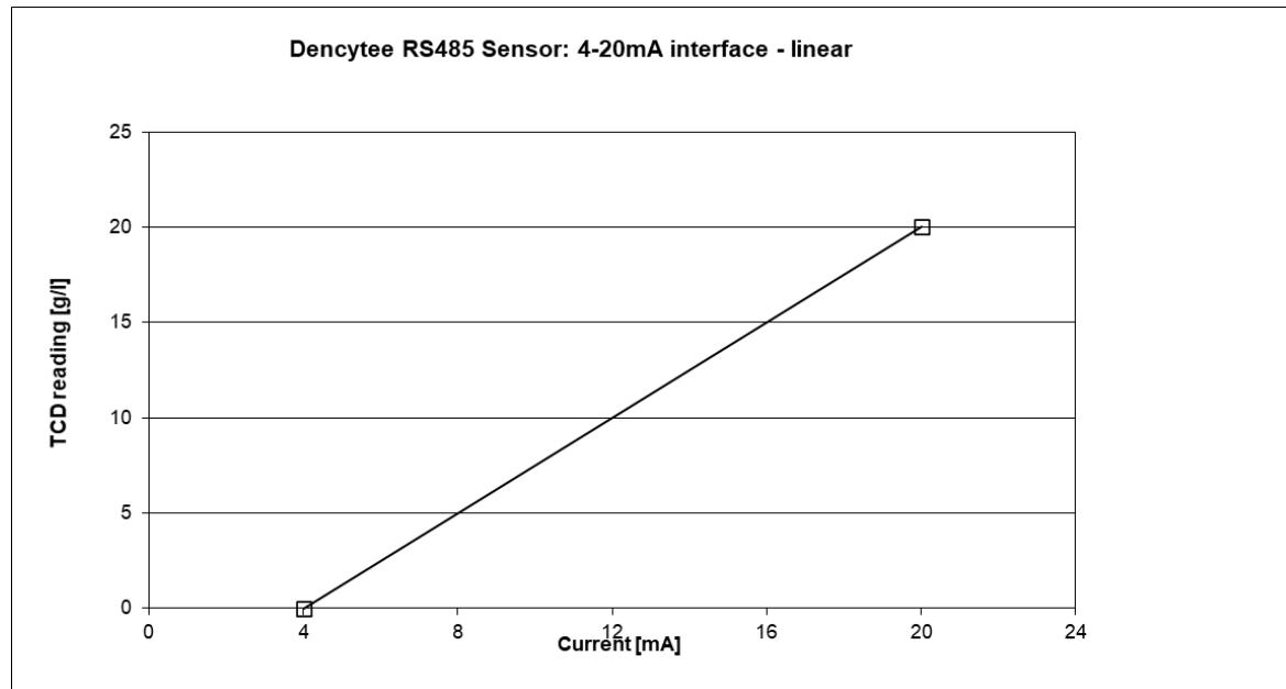
Figure 14 Example of linear 4-20mA output characteristics
