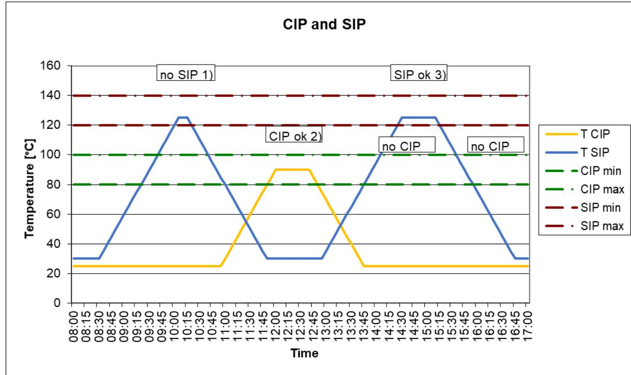
Figure 16 Definition of CIP and SIP cycles
