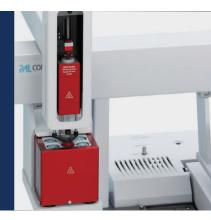
Hamilton offers a headspace syringe featuring a unique plunger designed specifically for the CTC PAL System Combi PAL®-xt gas chromatography (GC) autosampler. The High Dynamic (HD) plunger is optimized for high-throughput, excellent reproducibility, and sets a new standard for headspace syringes.
