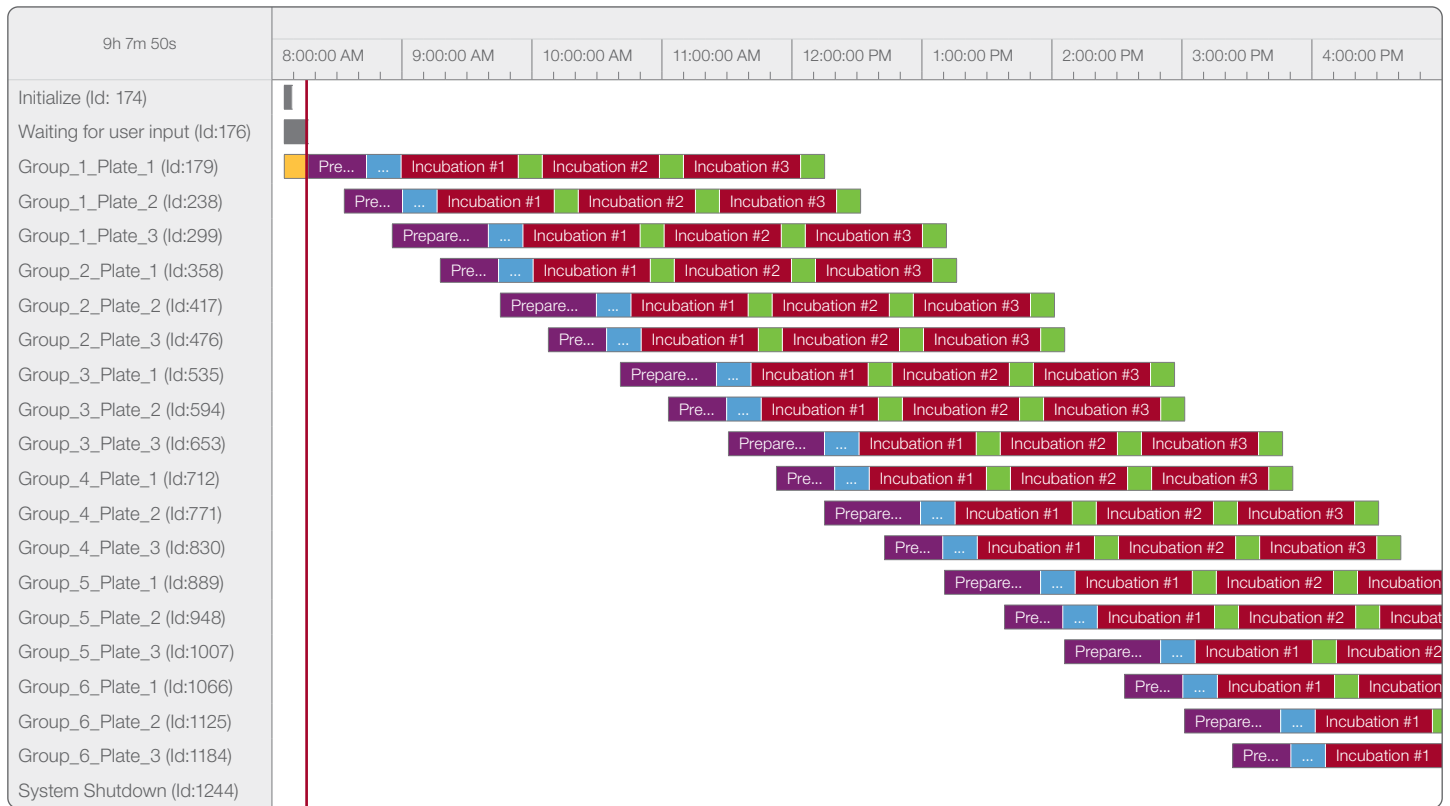
Figure 2. High-throughput automated parallel processing of ELISA plates.
